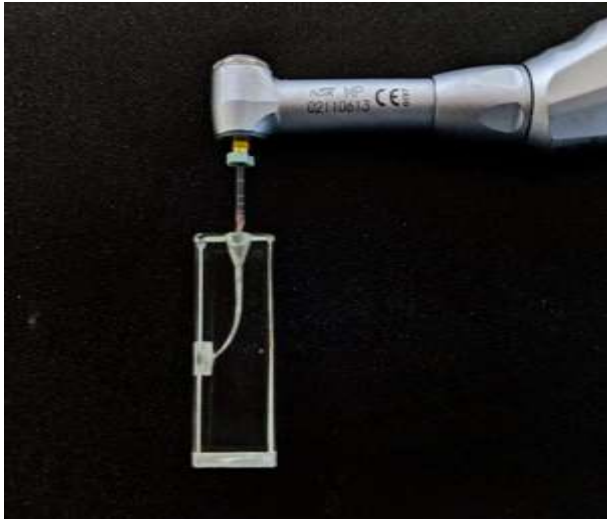
Figure 1: NiTi files subjected to rotary cycles in simulated acrylic canals of 45°
