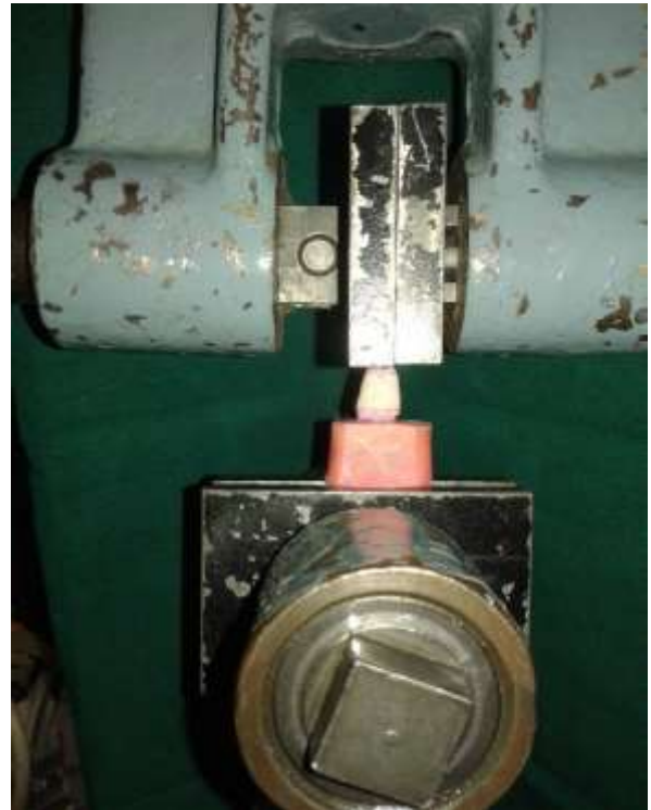
Fig.1: Ten Maxillary first premolars mounted in Acrylic supported by Dental Plaster.
