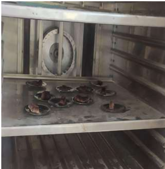
Fig. 2. Photographic image showing the moisture content of the coconut samples that were determined using a hot air oven.
