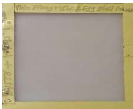
Fig. 2. Plain epoxy & hardener(10:1) 15% egg shell powder preparation mixture formed into plates on mica sheet (300x300x3mm) and folded by hand layup method.
