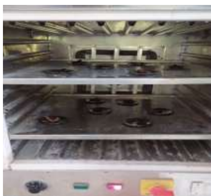
Fig. 2. Photographic image showing the moisture content of the coconut samples that were determined using a hot air oven.
