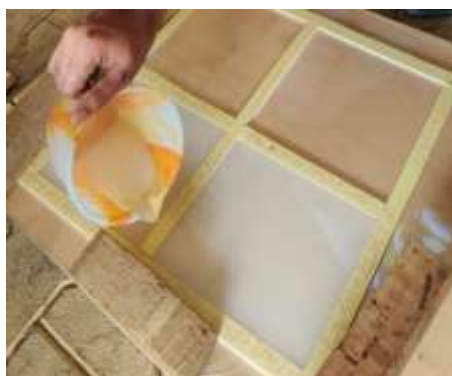
Fig. 2. Plain epoxy & hardener(10:1) with 5% egg shell powder mixture formed into plates on mica sheet (300x300x3mm) and folded by hand layup method.
