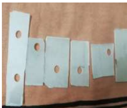
Fig. 4. CNC machined Plain epoxy + 5% egg shell powder 16 samples drilled by 8mm drill bit.
