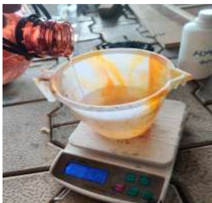
Fig. 1. Plain epoxy & hardener(10:1) mixture formed into plates on mica sheet (300x300x3mm) and folded by hand layup method.
