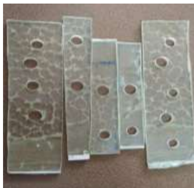
Fig. 3. CNC machined Plain epoxy 16 samples drilled by 8mm drill bit.
