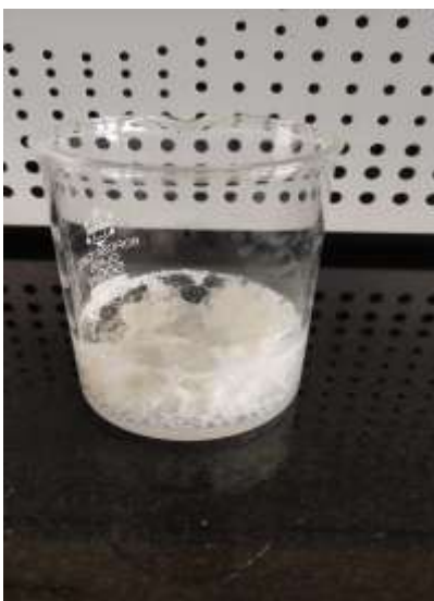
Fig. 5. Confirmation of Calcium ion in HAP synthesized from egg shell
