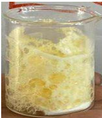
Fig. 4. Confirmation of Phosphate ion in chemically synthesized HAP
