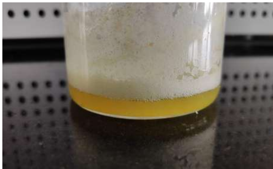
Fig. 6. Confirmation of Phosphate ion in HAP synthesized from egg shell
