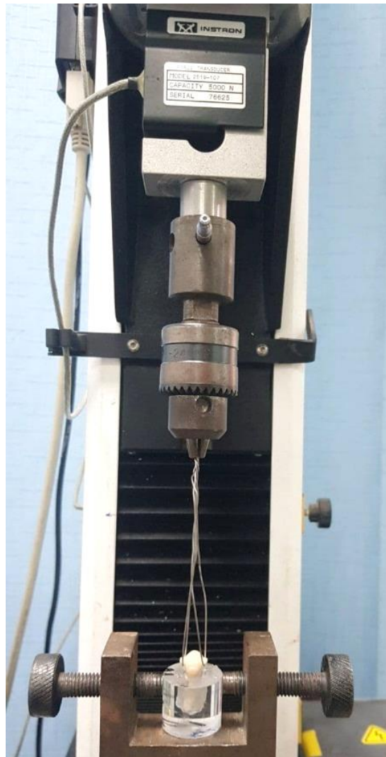
Figure (5): Pulling out the crowns using specially designed loop in a universal Testing Machine
