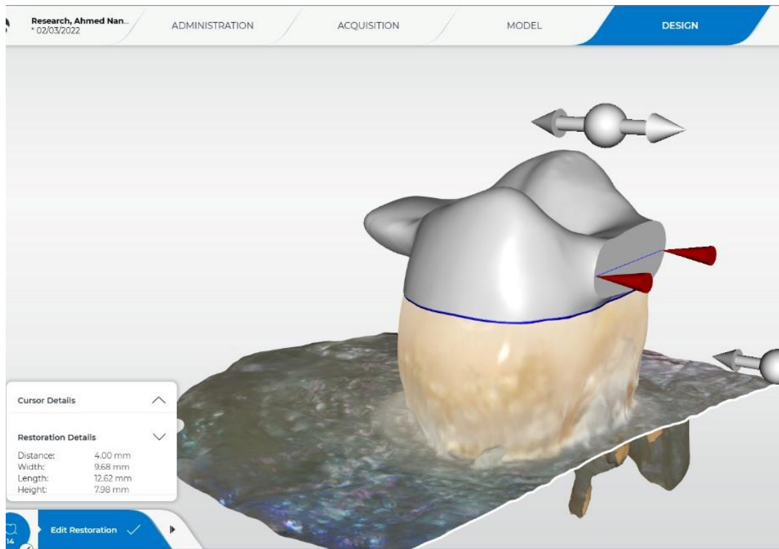
Figure (2): Virtual model of the two lateral projections included to the endocrown design. Height dimensions (A) width dimensions (B)
