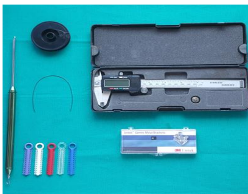
Fig -2: vernier calliper used for measuring tooth movement
