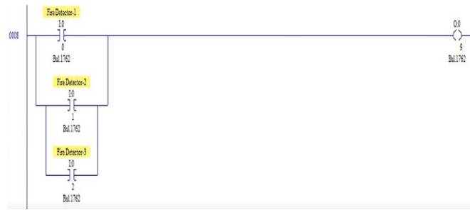
FIGURE 5. PLC PROGRAM PART 3
