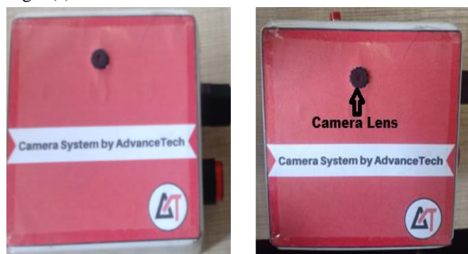
Fig. 3(a) Camera Module used to capture sky images
