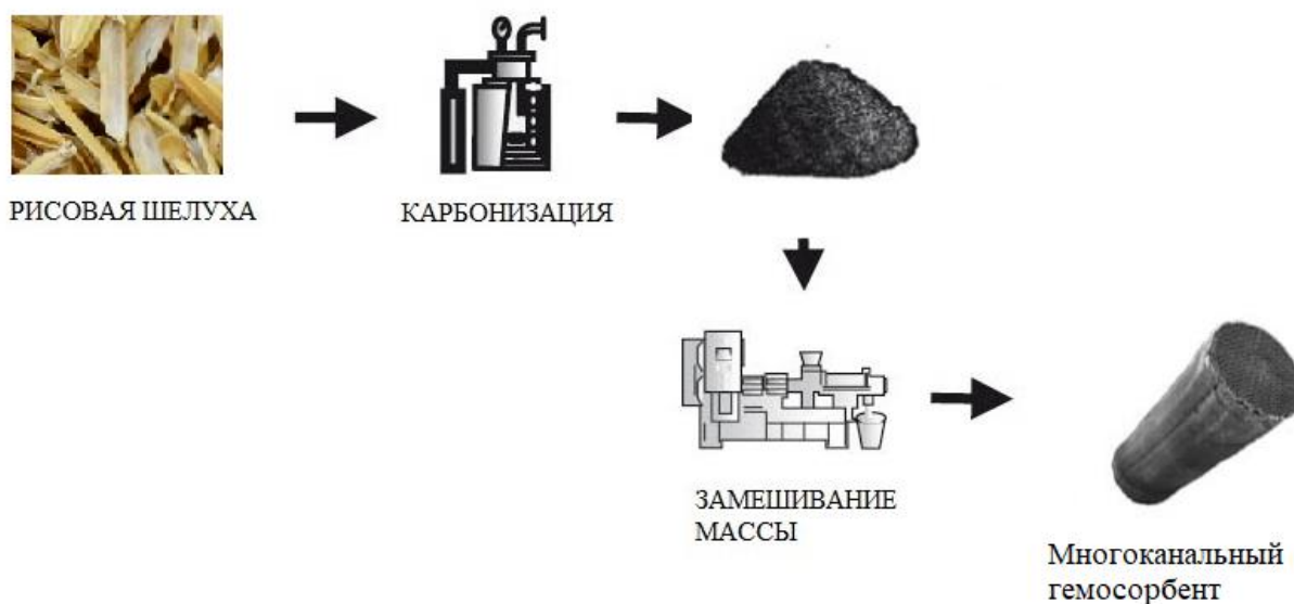
Figure 2 – technological operations for obtaining a carbon monolith of direct flow with a multi-channel structure
