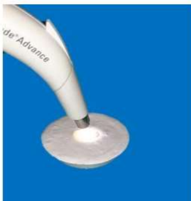
Figure 9 : Probe of the Easysshade was held perpendicular against the marked middle third of the sample
