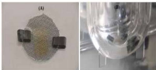
Fig.2. A) Watch glass covered with nylon wire mesh and B) Modified type 5 dissolution apparatus
