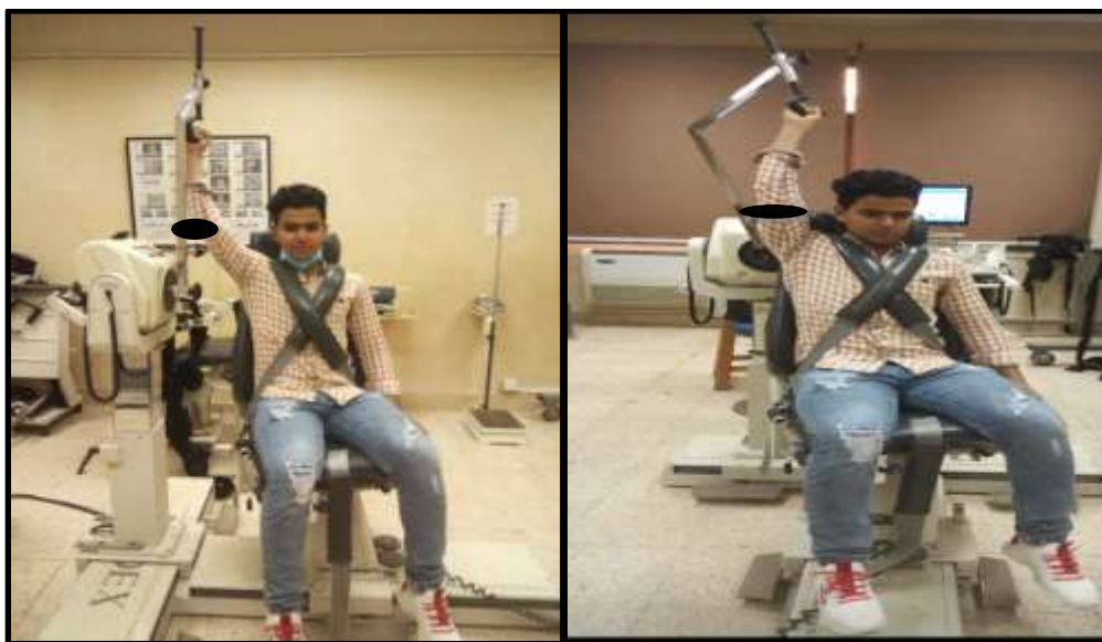
Fig. (1): Isokinetic testing of shoulder flexors performance. Fig. (2): Isokinetic testing of shoulder abductors performance
