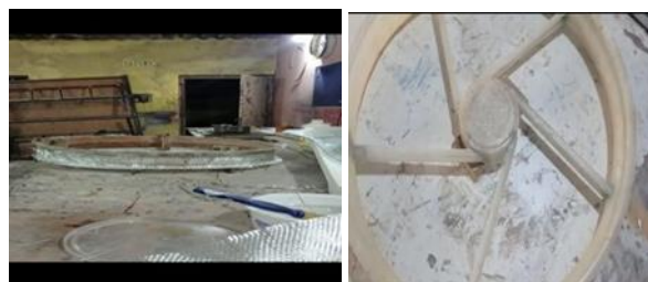
Fig. 2. Pasting carbon fiber to the rim and final product
