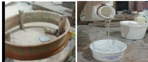
Fig. 1. Model preparation and adding epoxy resin
