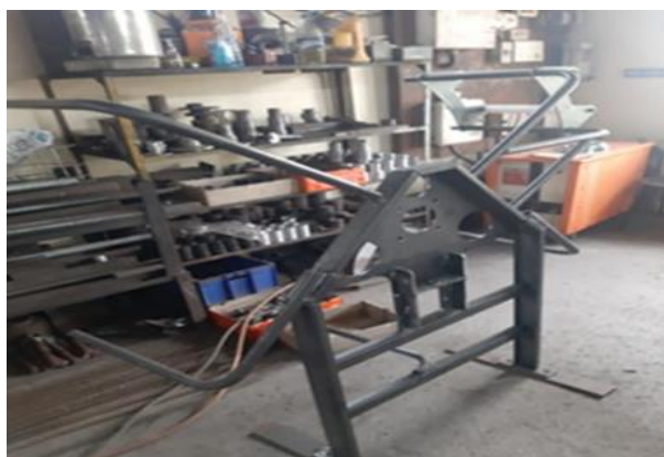
Fig.6: Support for mounting hose reel
