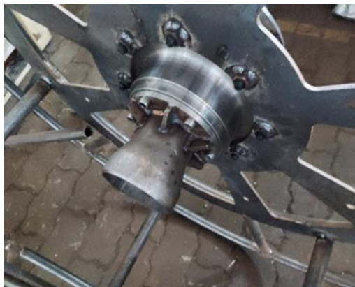
Fig.8: Hub Assembly with reel
