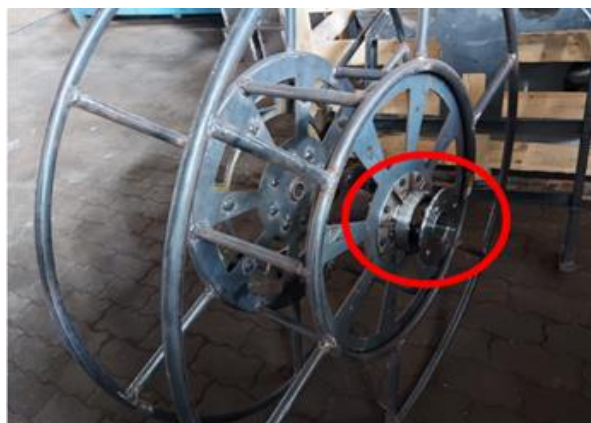
Fig. 7: Flange Assemblies installed on reel
