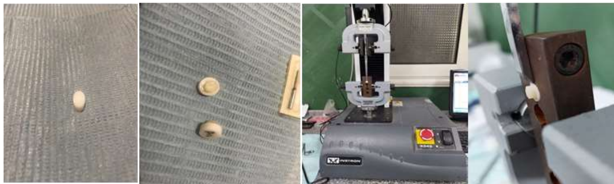
Fig. 1 Steps of sample preparation, translucent zirconia disc, after surface ttt and adhesive type application, repair composite building then loaded to Instron device for shear testing
