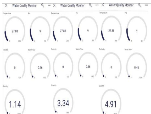
Fig. 5 IoT monitored Data through Blynk App in Domestic
