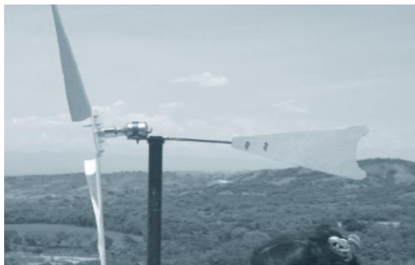
Figure 5. A weathervane that is mounted to the platform and secured to the iron bar.
