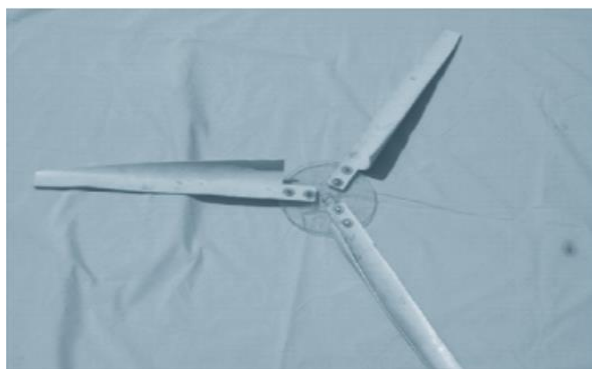
Figure 7. Final design of the blades made with PVC tube.
