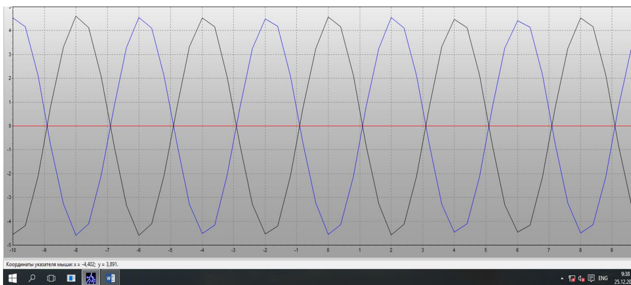
Figure 8. Graphic representation of synchronous motor phase currents when phase C is disconnected
