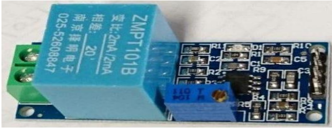
Figure 3. Overview of a voltage sensor that detects phase voltages.
