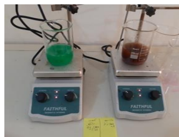
A. Preparation of NiCl 2 ·6H 2 O with cinnamons. B. Preparation of NiCl 2 ·6H 2 O with ginger solution. C. Prepare NiCl 2 ·6H 2 O with a solution of turmeric.
