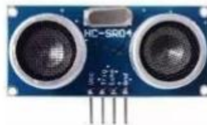
Fig. 4 HC-SR04 Ultrasonic Sensor
