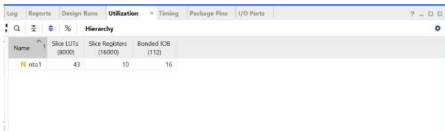
Figure 10. Device Utilization of proposed-2 Multiplier
