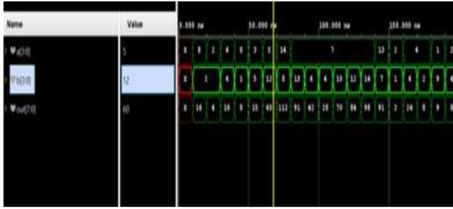
Figure 7. Simulation result of 4 X 4 Propose-2 Multiplier
