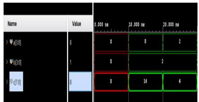
Figure 6. Simulation result of 4 X 4 Propose-1 LUT based Multiplier
