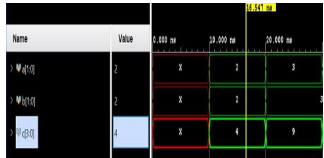
Figure 5. Simulation result of 2 X 2 LUT Based Multiplier
