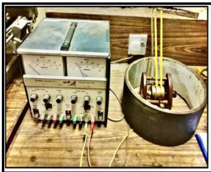
Fig. (2): Thermal conductivity apparatus (Lee disc)
