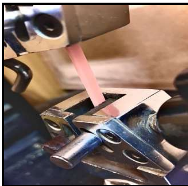
Fig. (4): The Specimen is subjected to tensile strength test
