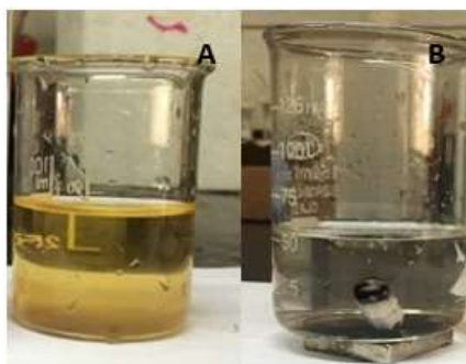
Fig. 3: Photographs of magnetic solid phase extraction steps: (A) before extraction, (B) magnetic separation
