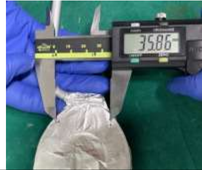
Figure 16 DPIcA measurement using calliper
