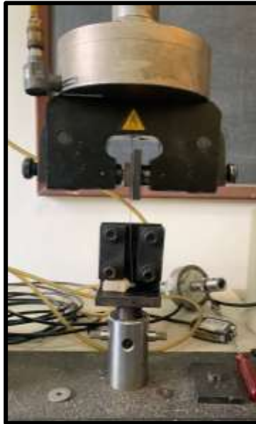
Fig.2 Evaluation of shear bond strength by Universal Testing machine
